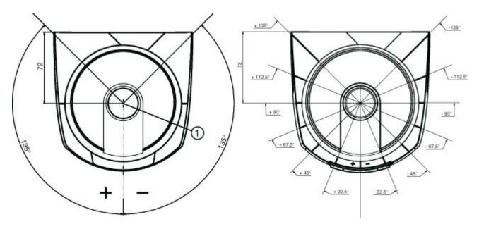
1 Reference point for distance measurement and protective field radius
