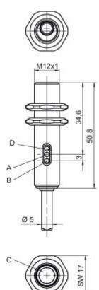
A Green LED B Yellow LED C Optical axis D Potentiometer
