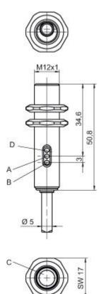
A Green LED B Yellow LED C Optical axis D Potentiometer
