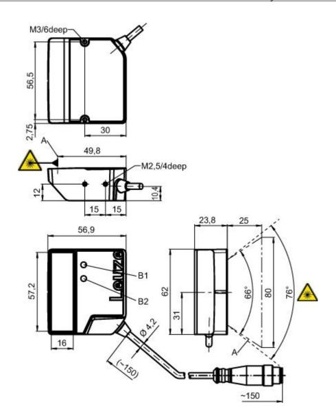
A Laser beam B1 Decode LED
