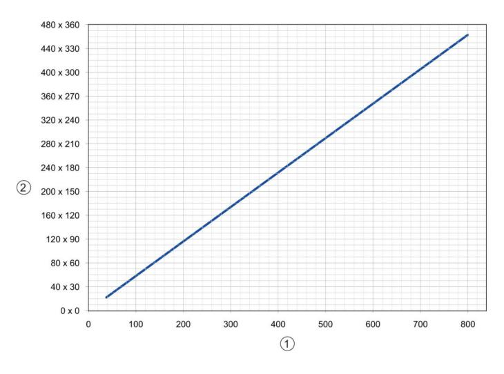
Camera distance [mm] Reading field: width x height [mm] 1 2
