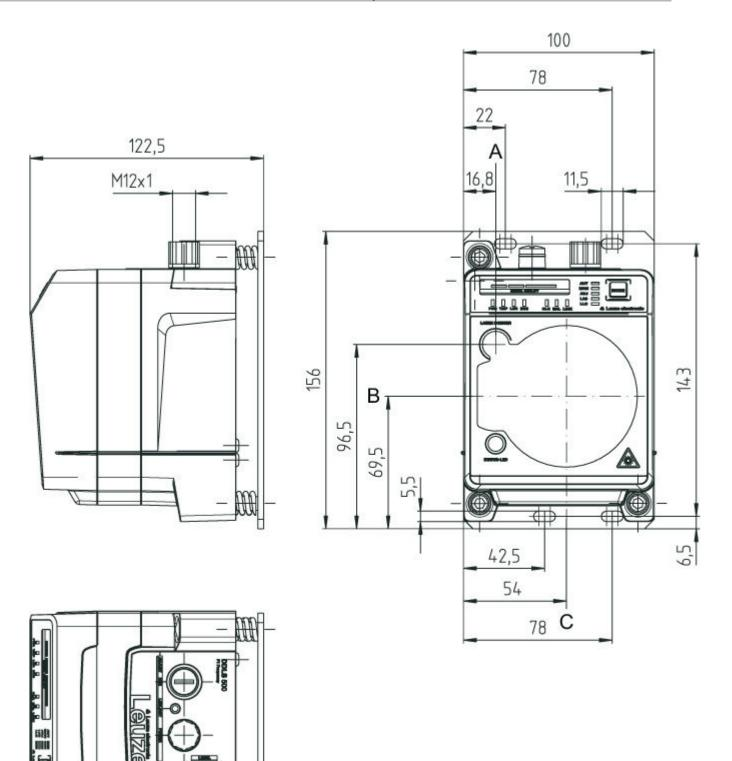
A Center axis of transmitter and alignment laser B Center axis of transmitter and receiver C Center axis of receiver
