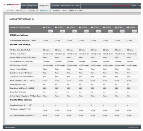
Figure 16: Modbus/TCP Settings Configuration Page
