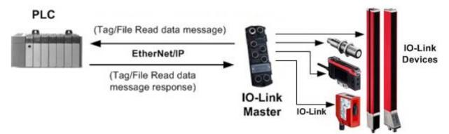
Figure 55: Read-from-Tag/File Tx Transfer Method
