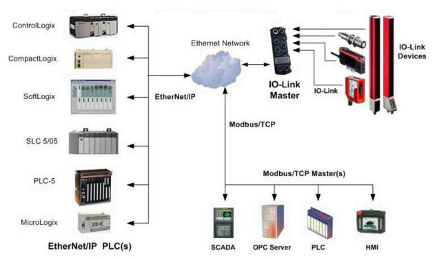
Figure 50: IO-Link Master Connectivity
