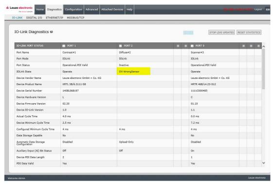
Figure 43: IO-Link device validation
