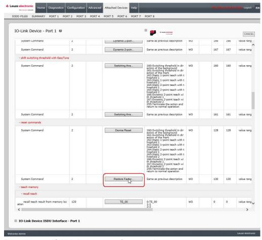
Figure 35: IO-Link device restore factory settings
