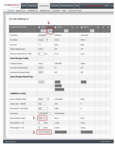
Figure 44: Upload device data for validation
