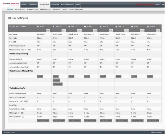
Figure 12: IO-Link Configuration Page
