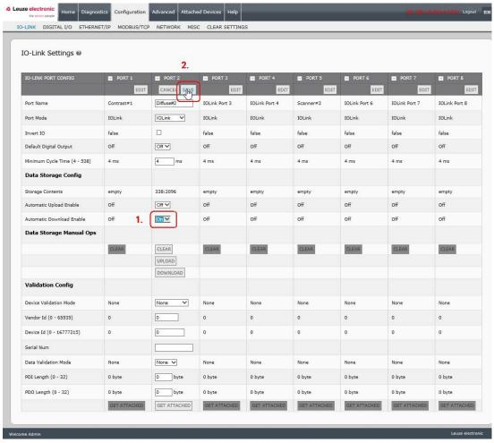
Figure 40: Data storage configuration
