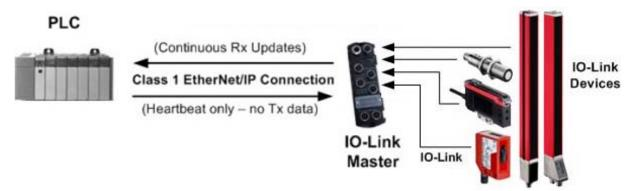
Figure 53: Class 1 Rx Transfer Method
