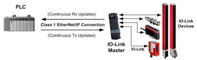
Figure 56: Class 1 Rx/Tx Transfer Method
