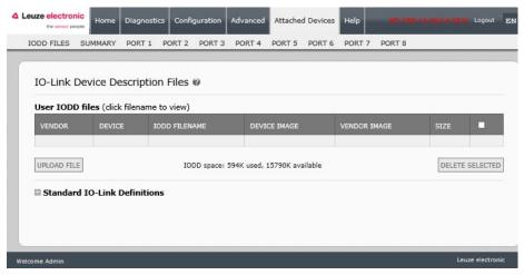
Figure 20: IO-Link Device Description files page
