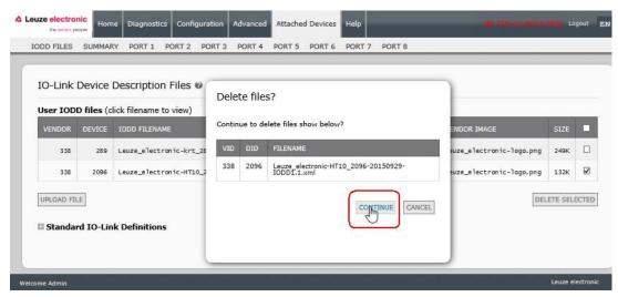
Figure 30: Confirm deleting of IODD files
