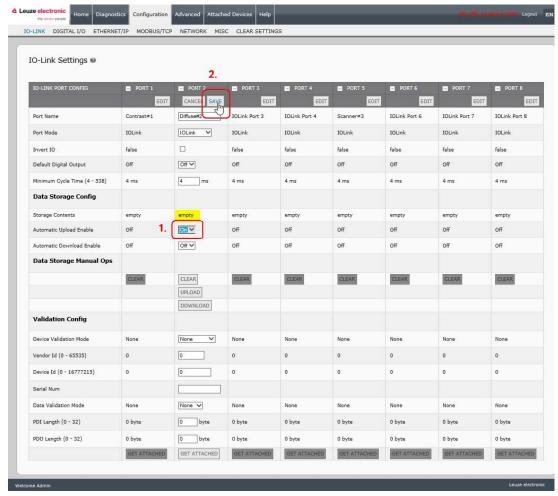
Figure 41: Activate automatic data storage upload
