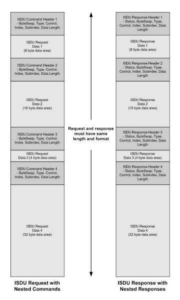
Figure 62: Example – Multiple Command ISDU Request/Response of Different Data Area Lengths
