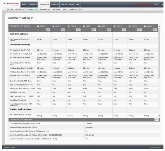
Figure 14: EtherNet/IP Settings Configuration Page
