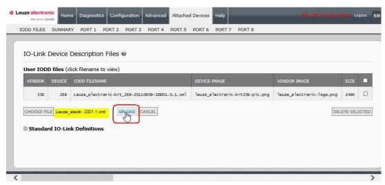
Figure 25: Unload IODD file
