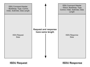
Figure 60: Single Command ISDU Request/Response
