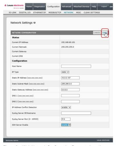
Figure 3: Web Network Configuration Page: static setting
