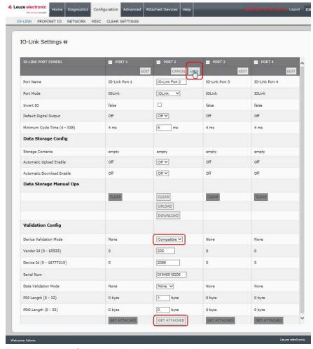
Figure 42: IO-Link device validation settigns
