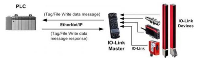
Figure 52: Write-to-Tag/File Rx Transfer Method
