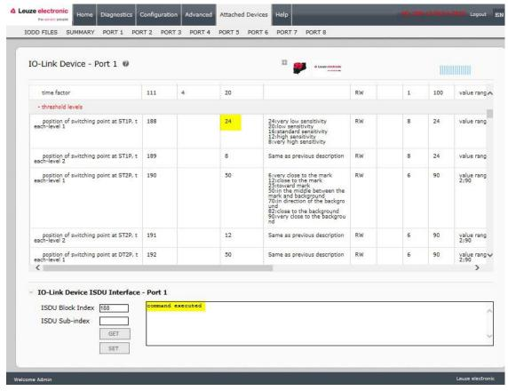
Figure 38: IO-Link iSDU feedback
