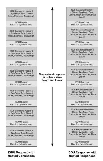
Figure 61: Example - Multiple Command ISDU Request/Response of Different Data Area Lengths
