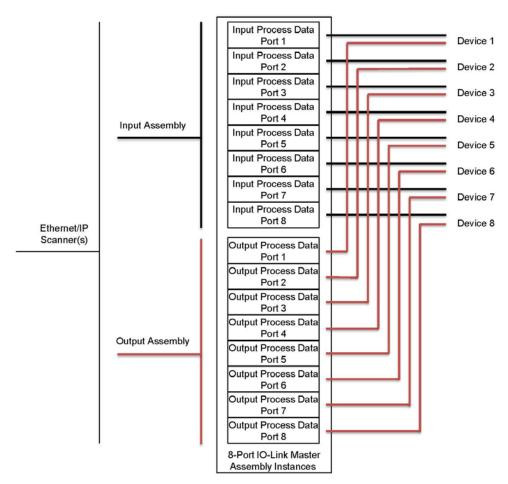
Figure 58: Overview of Assembly Interface, 8-Port 10-Link Master Assembly Instances
