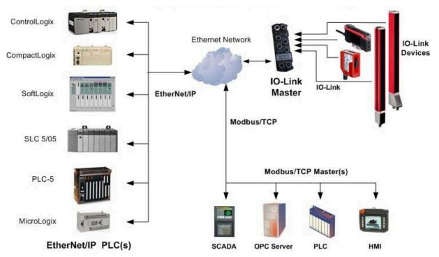
Figure 59: Modbus/TCP to IO-Link
