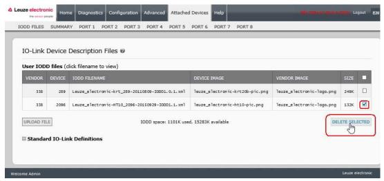
Figure 29: Deleting IODD files
