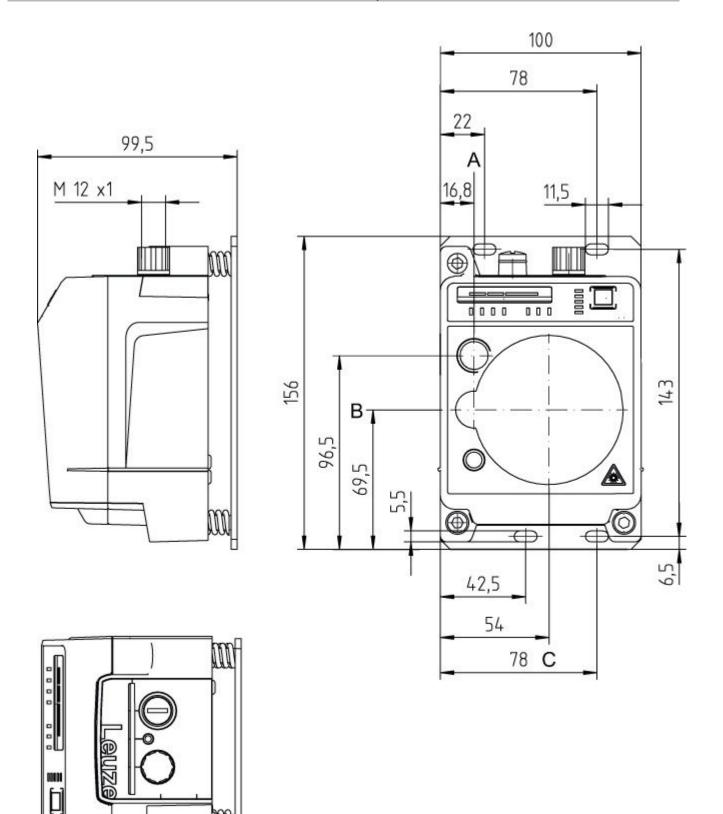
A Center axis of transmitter and alignment laser B Center axis of transmitter and receiver
