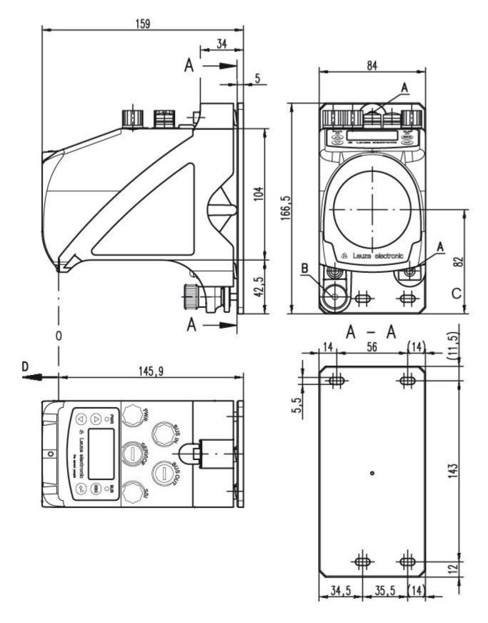
A M 5 screw for alignment
