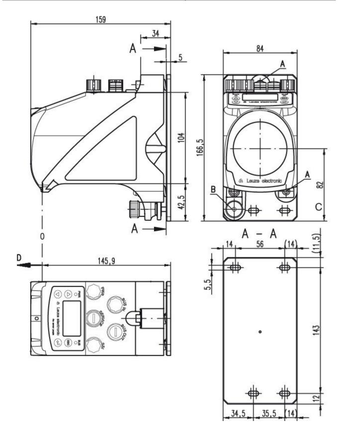
A M 5 screw for alignment
