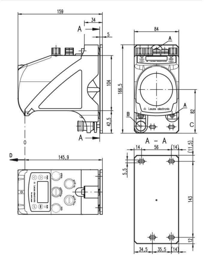
A M 5 screw for alignment
