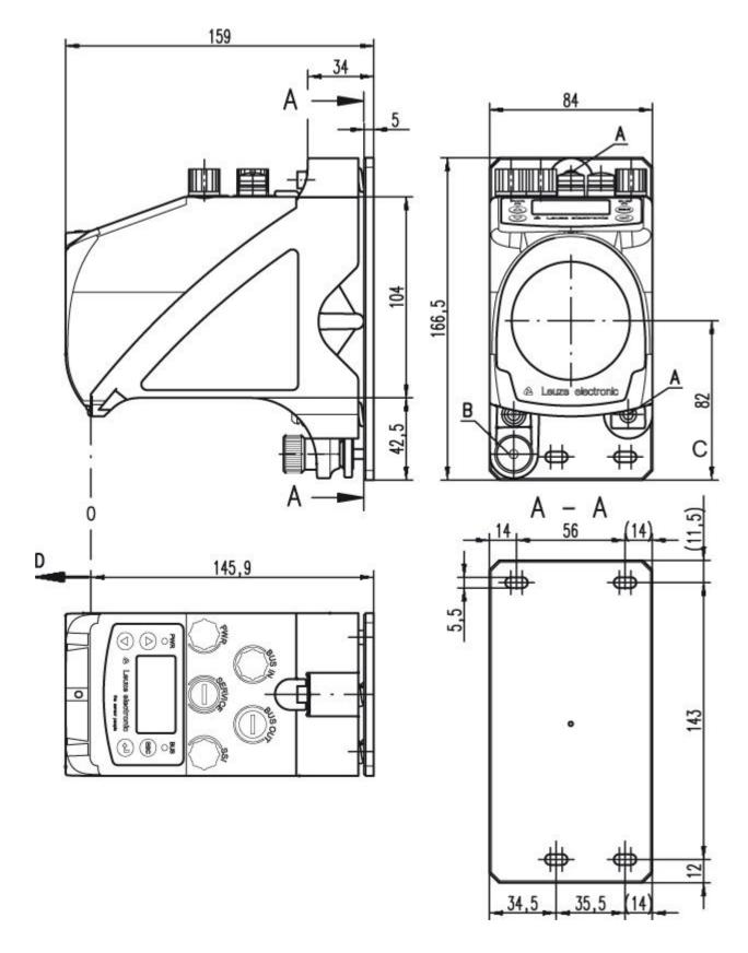
A M 5 screw for alignment
