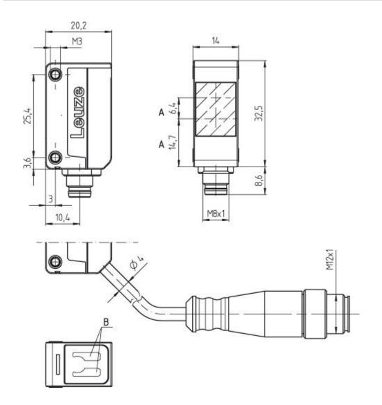
A Optical axis B Indicator diode
