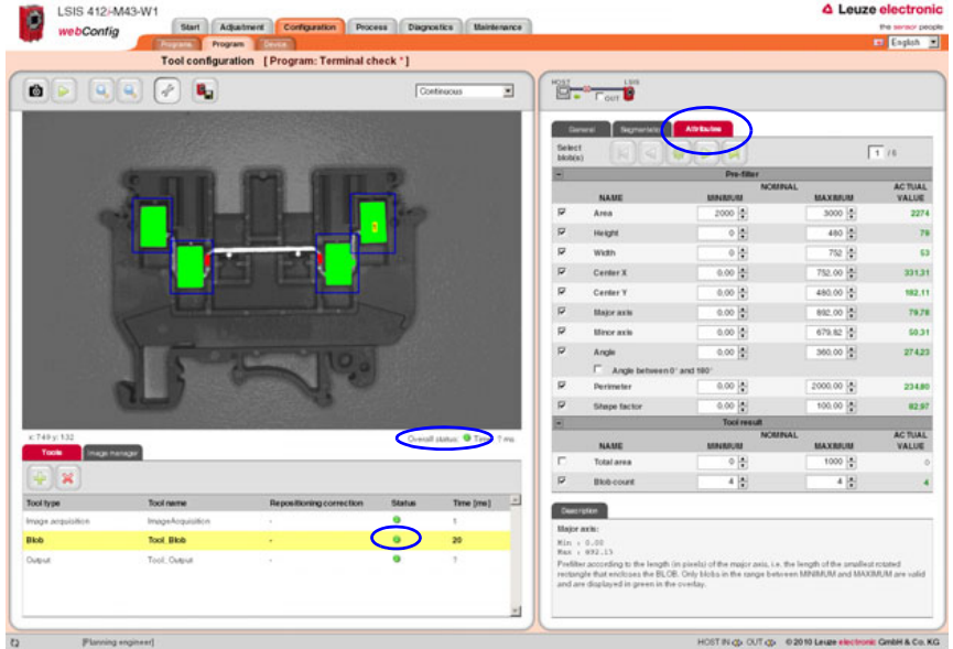
Figure 4.9: Evaluating object attributes: part OK
