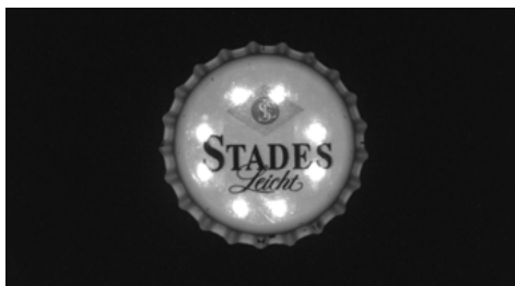
Figure 4.12: Vertical camera alignment – maximum reflections
