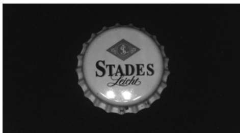
Figure 4.13: Inclined camera alignment with all four illumination quadrants active – better, but reflections still visible in one quadrant
