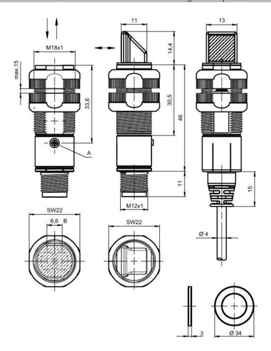
B Optical axis A Indicator diode
