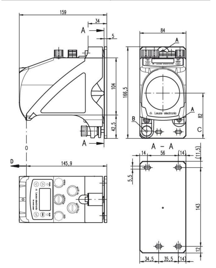
A M 5 screw for alignment
