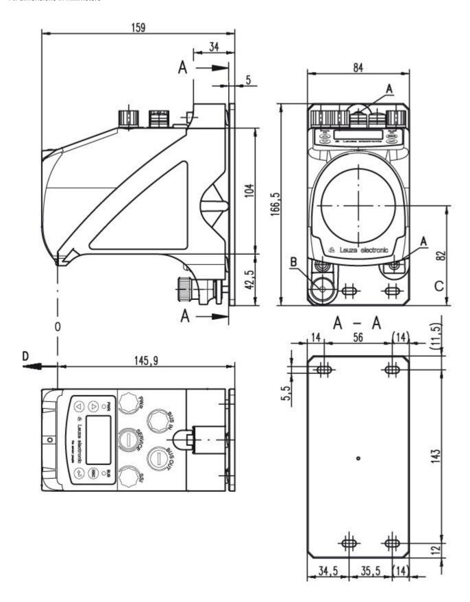
A M 5 screw for alignment
