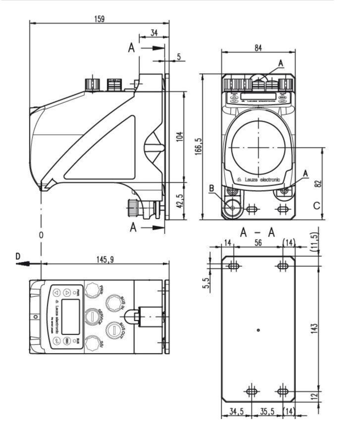
A M 5 screw for alignment
