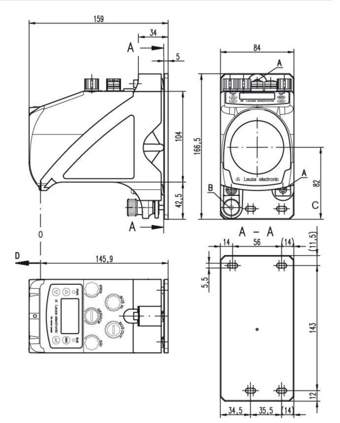
A M 5 screw for alignment
