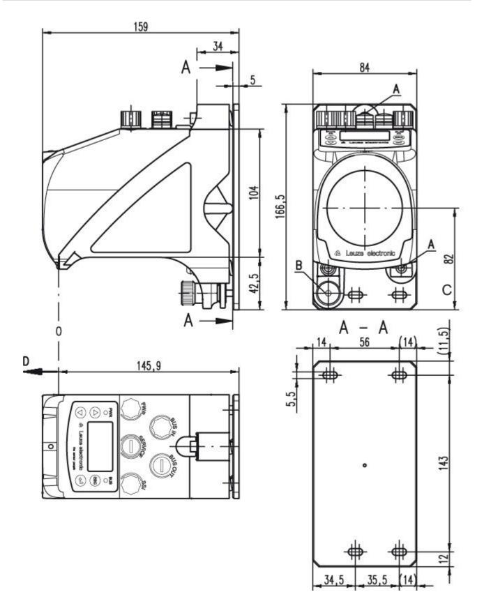
A M 5 screw for alignment
