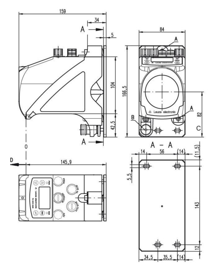
A M 5 screw for alignment
