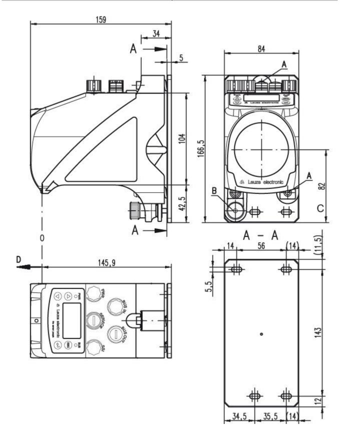
A M 5 screw for alignment
