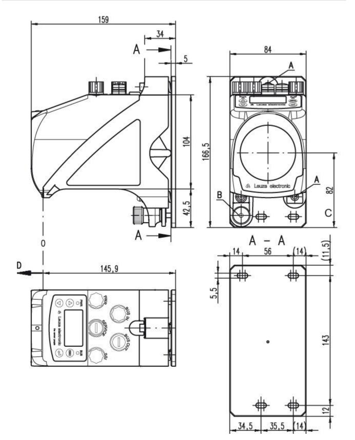
A M 5 screw for alignment
