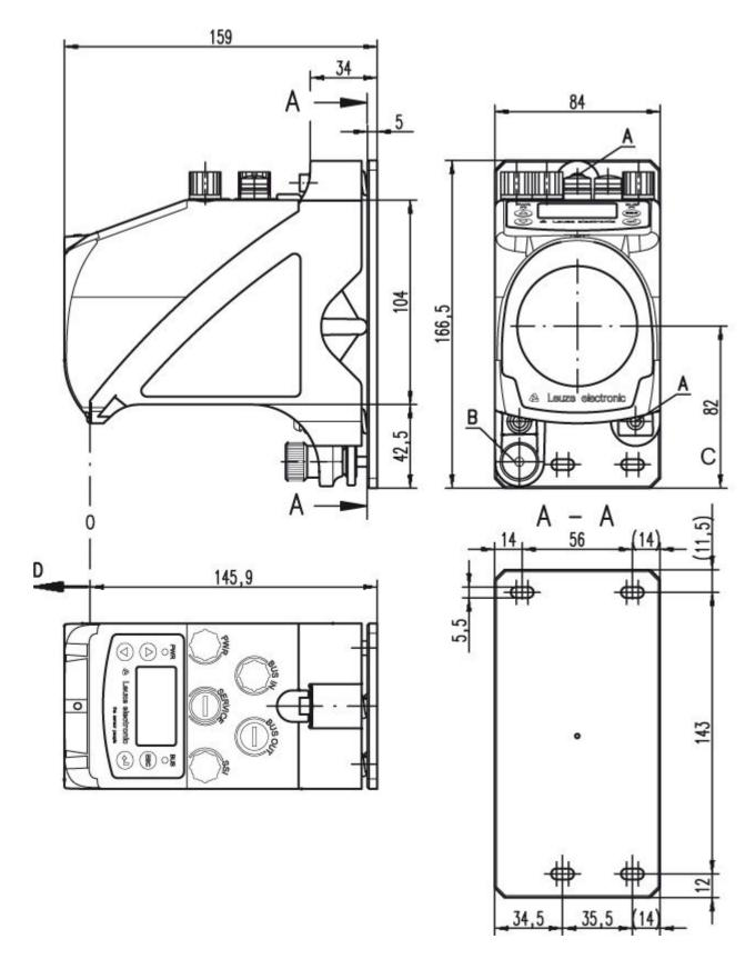
A M 5 screw for alignment
