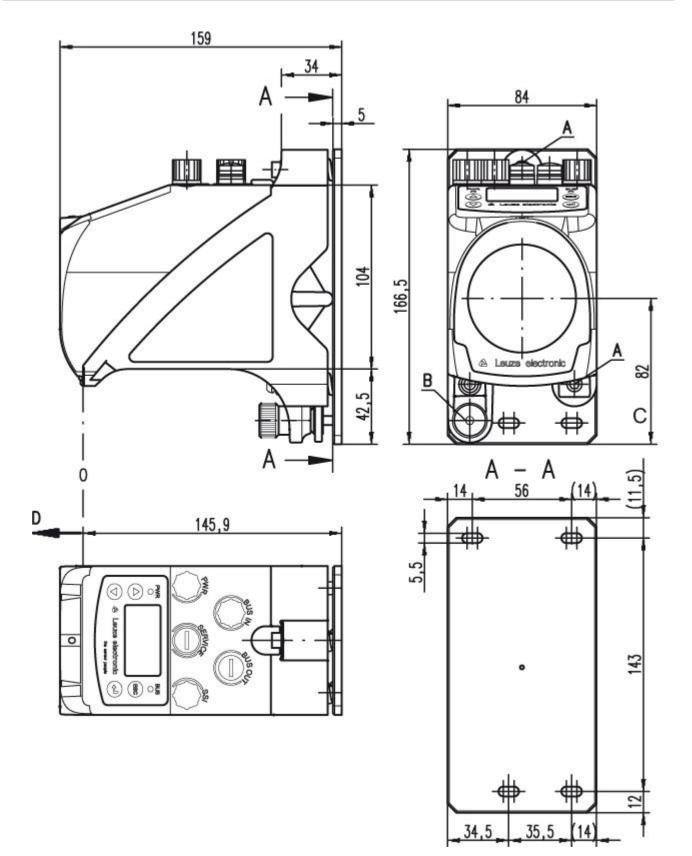
A M 5 screw for alignment
