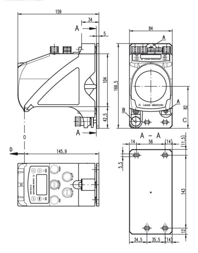
A M 5 screw for alignment
