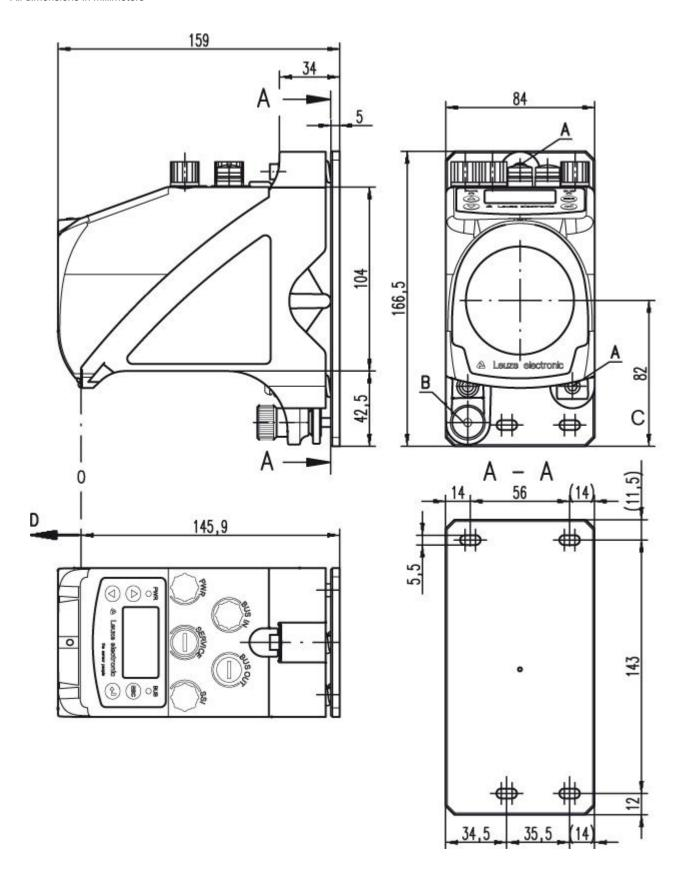
A M 5 screw for alignment
