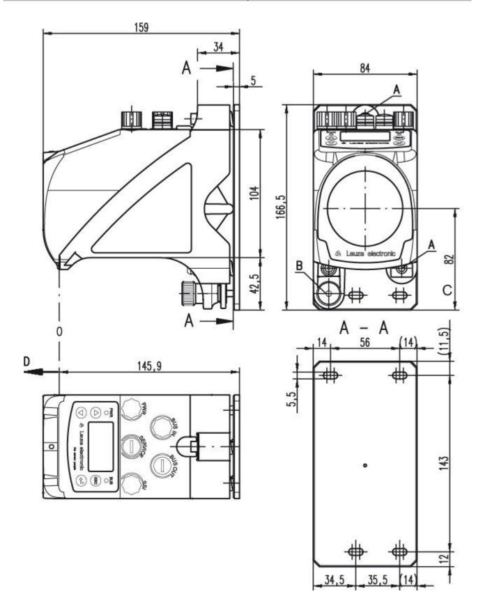
A M 5 screw for alignment
