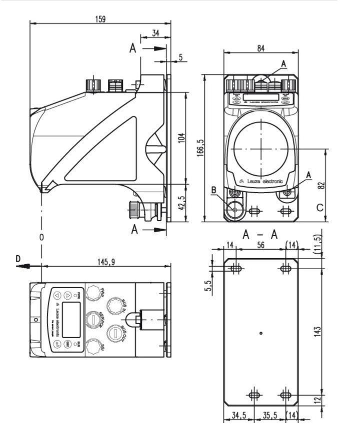
A M 5 screw for alignment
