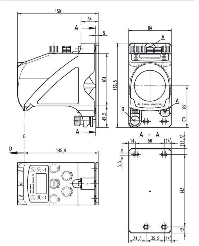
A M 5 screw for alignment
