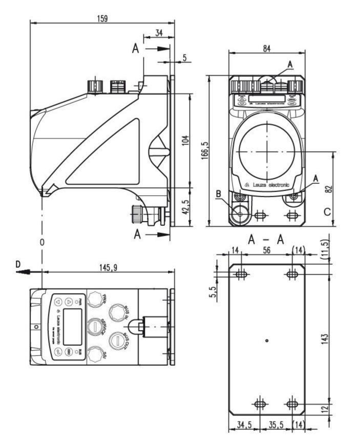
A M 5 screw for alignment
