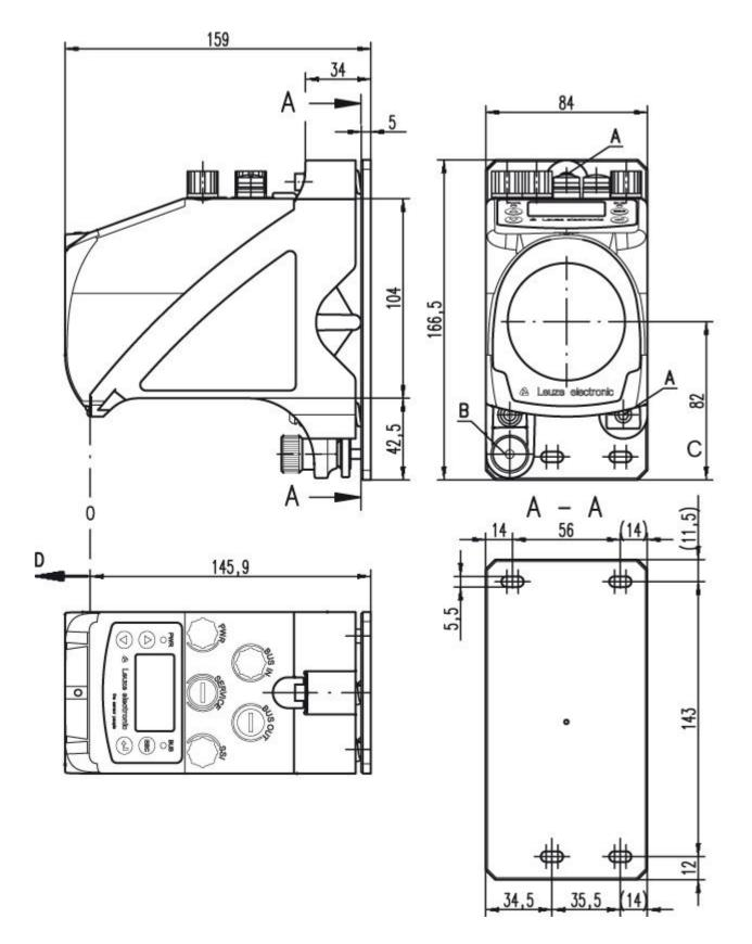
A M 5 screw for alignment
