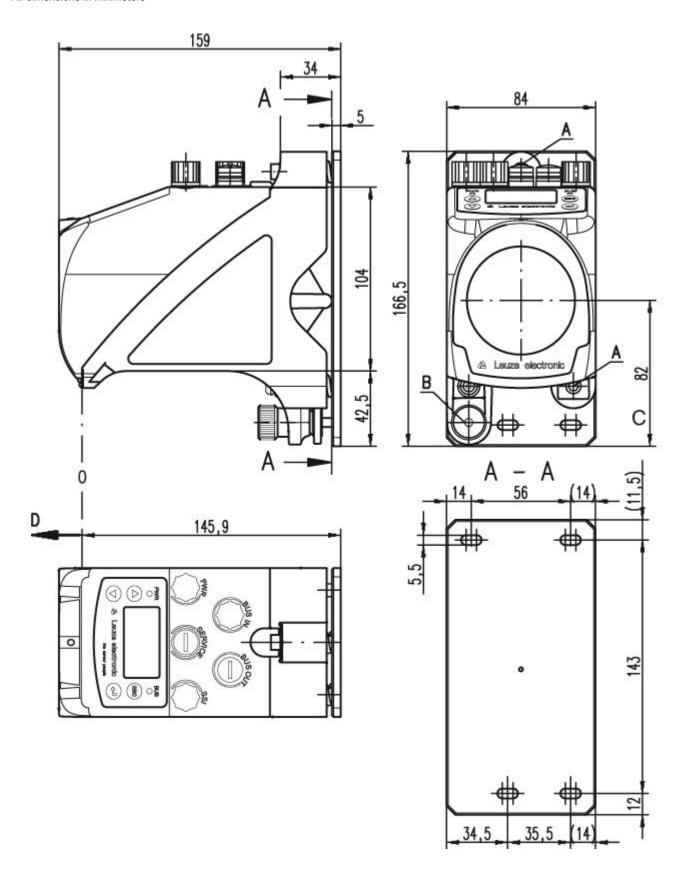
A M 5 screw for alignment
