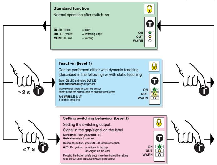
= function lockable through constant application of  $U_B$  on the teach input (for devices with teach input only)
