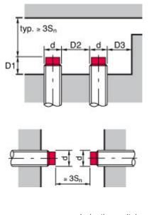
Inductive switch a b Standard measuring plate
