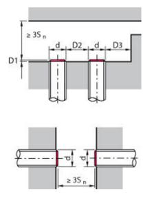
a Inductive switchb Standard measuring plate
