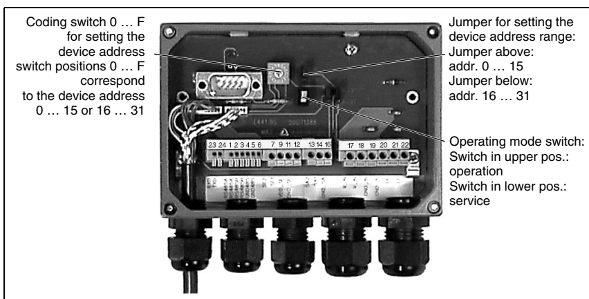
Figure 7.1: Configuration elements in the MA 2
