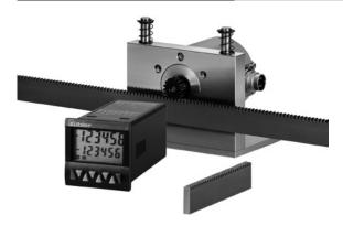
Measuring system with mobile encoder holder, mounted on springs, (with rack and pinion) for an optimum contact pressure and protection of the encoder shaft.
