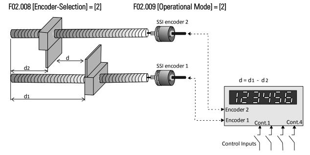
Both encoder inputs are connected to SSI encoders and the unit calculates the differential position of both encoders. The encoders may have different resolutions and can operate at different Baud rates and individual scaling. The result of the calculation (difference) can once more be converted to the desired engineering units by means of the final scaling parameters.
