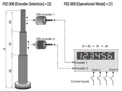
Both encoder inputs are connected to SSI encoders and the unit calculates the sum of positions of both encoders. The encoders may have different resolutions and can operate at different Baud rates and individual scaling. The result of the calculation (sum) can once more be converted to the desired engineering units by means of the final scaling parameters.
