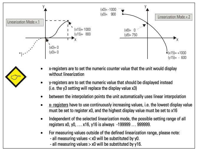
The diagram below explains the difference between Linearization Modes 1 and 2:
