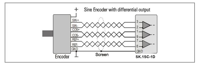
With sensors using single-ended outputs, the sensor signals SIN, COS and REF are connected to the corresponding input pins. The inverted inputs of the unit can be connected <u>either</u> to the mean voltage output Vm (pin 8) of the unit <u>or</u> to a corresponding voltage reference of the sensor itself.
