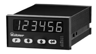
Frequency display for demanding applications, with two individually scalable encoder inputs, in each case A, /A, B, /B for count frequencies up to 1 MHz per channel (also for single channel use).
