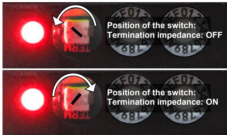
Figure 16 Position of Switch S3
