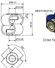
radial: max. ±3 mm angular: ± 12° 3000 rpm max. 200 Ncm zinc-plated polyurethan 85 g
