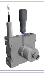
By tightening (approx. 2 Nm) the inner radial screw with a 2.5 mm hex wrench the encoder shaft will be clamped to the sensor mechanics and
